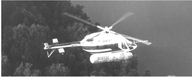
Figure 1. Helicopter with inflated ballonet
