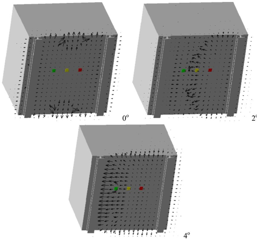
**Figure 9: Velocity distribution in plane near bottom,  $t=0.015s$  after start motion.**
