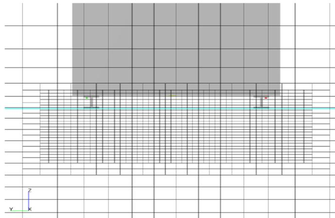
**Figure 6: The CFD mesh with local adaptation near impact region**
