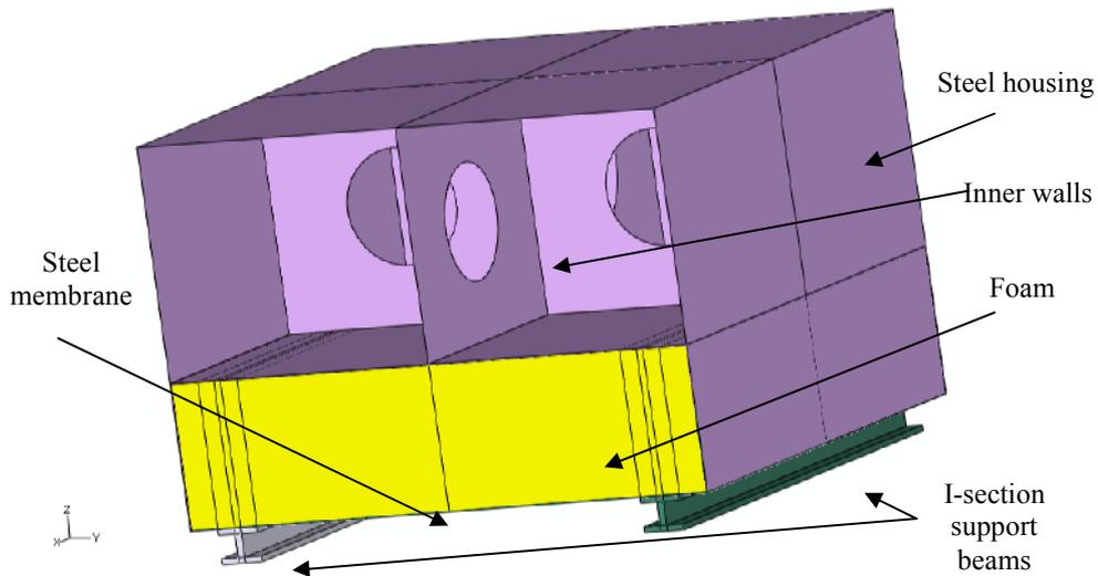
Figure 1: Components of testing drop-test structure
