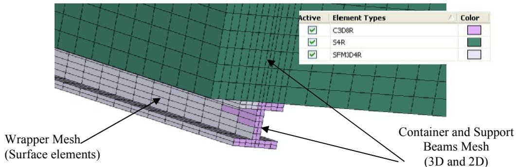
**Figure 4: Wrapper mesh defined for the container surface**
