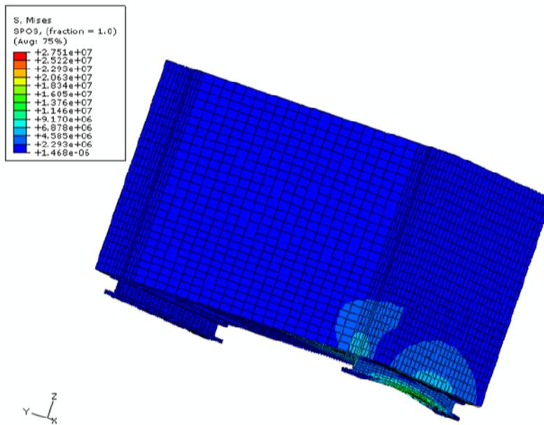
Figure 12: Deformation of support beams at first moments of container collision with water (deformation scalar factor 100)
