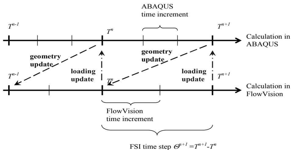
**Figure 6.1: FSI time step for FlowVision and Abaqus**
