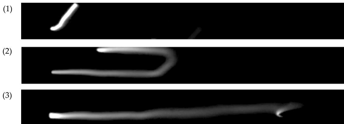
Figure 4. Photos of the discharge channel in the supersonic flow: (1,2) launch and (3) stable operation.
