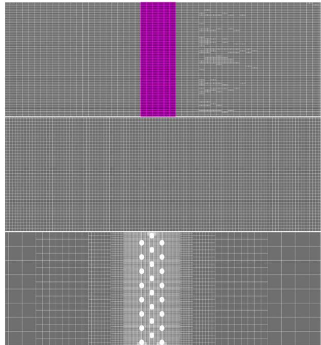
Figure5 Computational grid (side view) (from top to bottom; Gap Model, porous, grid resolved)
