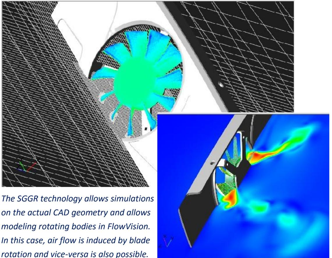
*The SGGR technology allows simulations on the actual CAD geometry and allows modeling rotating bodies in FlowVision. In this case, air flow is induced by blade rotation and vice-versa is also possible.*
