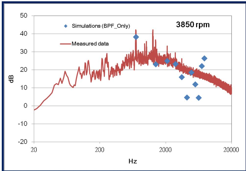
*The above graph illustrates comparison of experimentally measured noise levels with the simulation results.*
